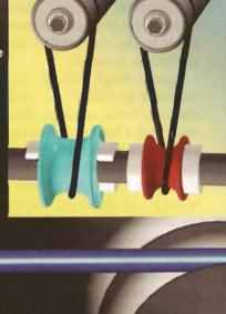
Don't get shocked Urethane usually insulates but some power transmission belts made of thermoplastic urethane embedded with conductive thermoplastic prevent static electric buildup caused by friction between belting and pulleys on conveyors and other machinery. With volume resistivity of 2 x 109 ohms-cm and a static decay rate less than 0.01 sec, this belt dissipates static better than varieties embedded with carbon and metal.
